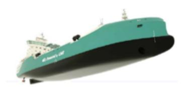
Capacity 10,000 m<sup>3</sup> Overall length 119.35 m Beam 20.5 m Gas/diesel-electric generation system Design by Ghenova Engineering
